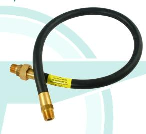
1/2" nominal size hose incorporating a union fitting. This hose does not conform to BS 669 as it does not incorporate a quick disconnect fitting, and therefore should not be used to connect domestic gas appliances in the UK.
