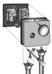
Remove the high limit cut out cover from the front of the thermostat and then by unscrewing the 3 screws remove the complete cover.
